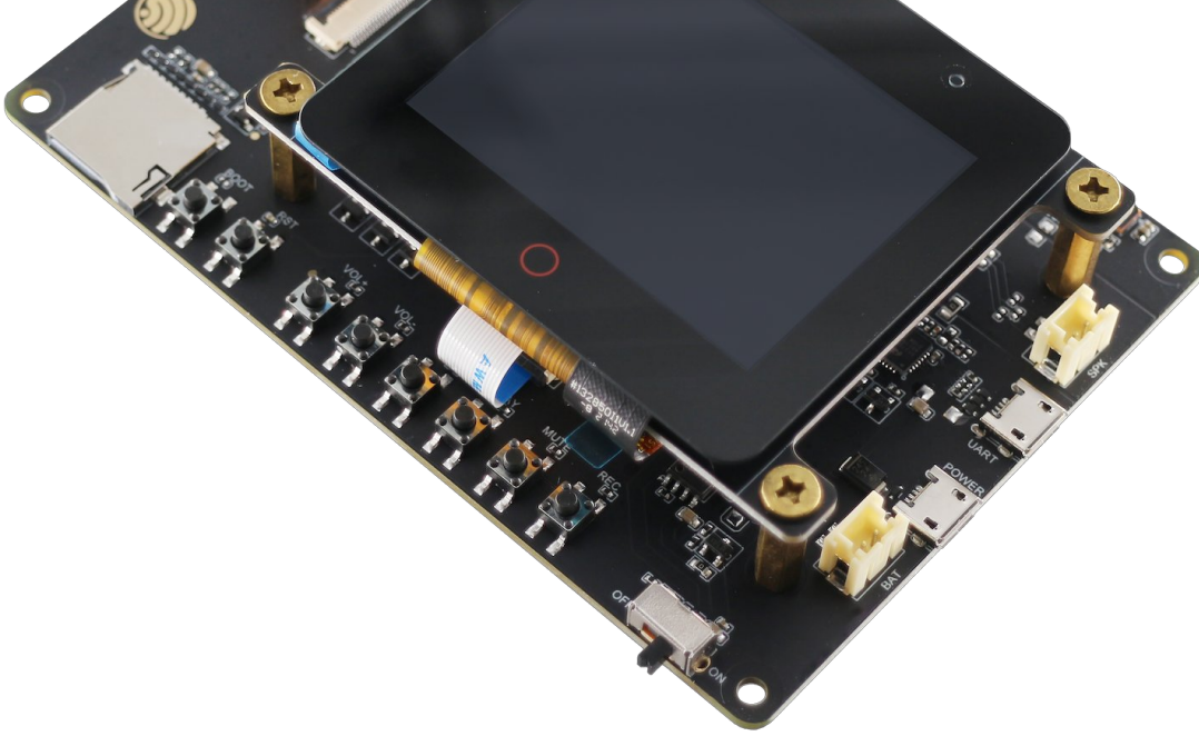
ESP32-S3-Korvo-2 V3.0 with ESP32-S3-WROOM-1 module
